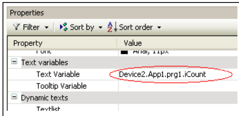
Fig.4-19: Example for using a data source variable in the properties of a visualization element
